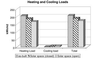
Figure 7: Annual energy loads for the simulated Mud-brick Building; with and without the solar space.
