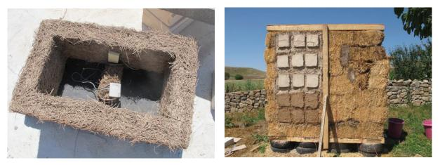
Figure 10. Academic research and experiments on building materials and their properties include the study of lightweight loam and pine-needles (left) and applying different types of mud plaster on straw bale walls to assess their durability (right).
