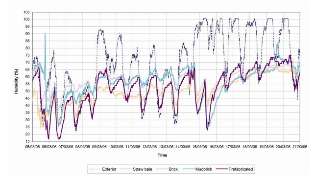
Figure 9b: Humidity chart to compare the behaviour of buildings constructed with four different wall materials, when heated intermittently with a room heater.
