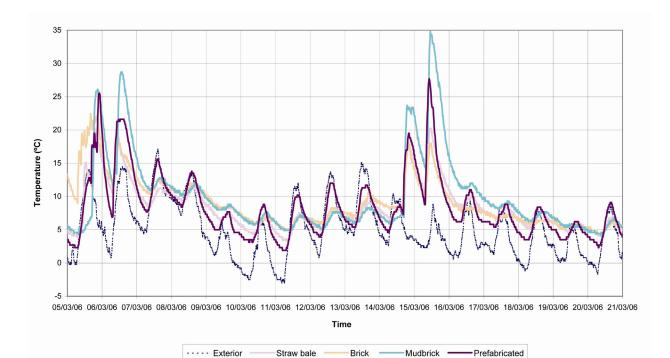
Figure 9a: Temperature chart showing the comparitive behaviour of buildings constructed with four different wall materials, when heated intermittently with a (coal & wood) room heater.
