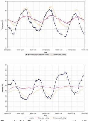
Figure 8a & b: Three-day temperature and humidity charts for straw bale and prefab buildings under unheated conditions
