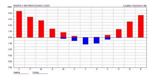
Figure 17: Monthly Heating/Cooling Loads of Basturk House with Hollow-Brick Walls.
