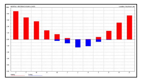
Figure 18: Monthly Heating/Cooling Loads of Basturk House with Mud-Brick Walls.
