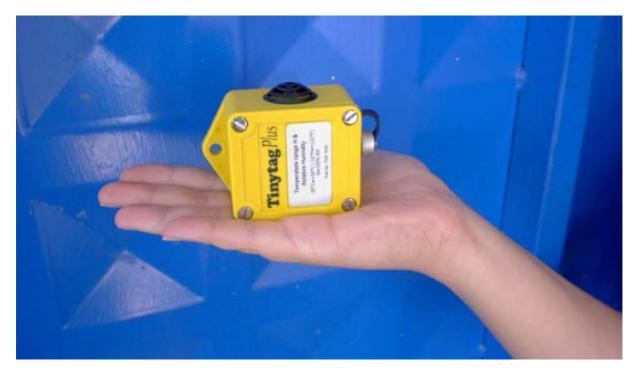
*Figure 5: Tinytag data logger with the sensor protected by a black spherical frame.*
