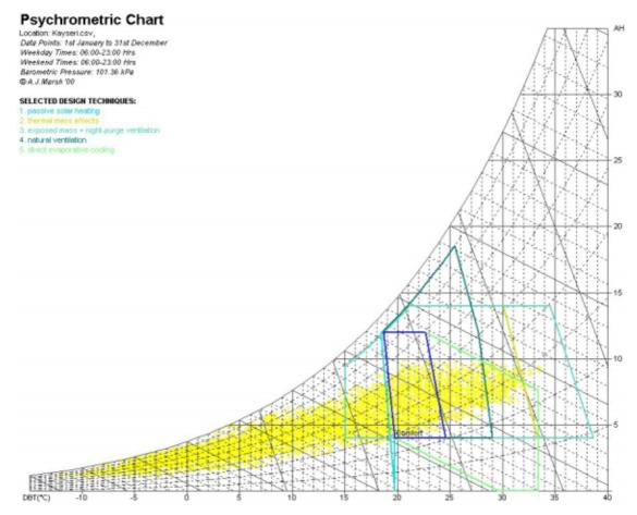
Figure 4: Hourly data for a Kayseri year plotted against thermal comfort zones on psychrometric chart (Source: Meteonorm and Weather Tool software).
