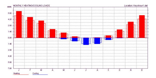
Figure 21: Comparative Graph Showing Monthly Heating/Cooling Loads of Basturk House with Hollow-Brick with and without Insulation. Hatched Bars Showing the loads with Hollow-Brick Walls with Insulation and Solid Bars Showing the loads with Hollow-Brick Walls without Insulation.
