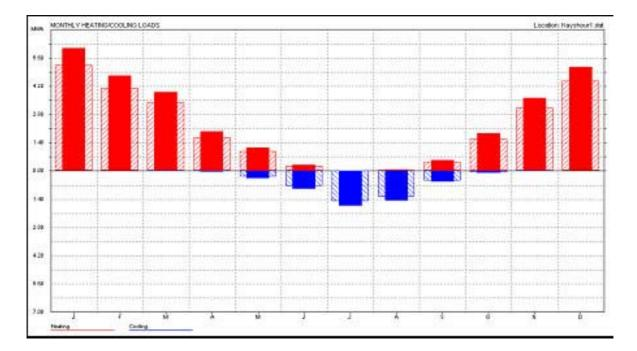
Figure 20: A Comparative Graph Showing Monthly Heating/Cooling Loads of Basturk House with Hollow- Brick and Mud-Brick Walls. Hatched Bars Showing the loads with Mud-Brick Walls and Solid Bars Showing the loads with Hollow-Brick Walls.
