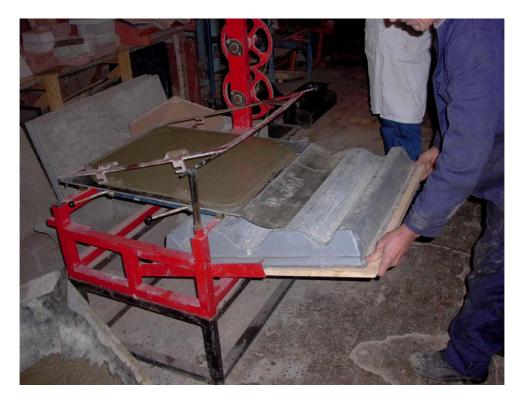
Figure 9. The plastic sheet on which the cement mix was poured can be pulled over the roof tile mould. Up to 20 moulds can be stacked for drying.
