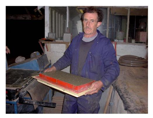
Figure 10. Moulds for the similar production of different types of roof tiles and paving slabs are also available.
