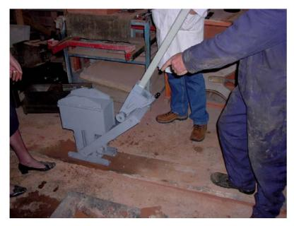
Figure 4. Pressure is applied to the mixture of clay, sand, cement and water in the Parry's Brick Press mould by means of a long handle.
