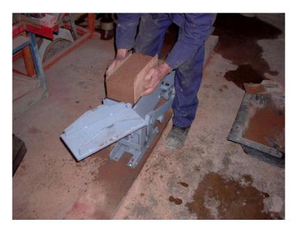
Figure 6. Once pushed up the brick can be taken out by holding it with two plywood pieces to avoid damage. The bricks are then stacked for drying.
