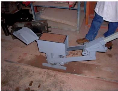
Figure 5. The lid of the brick press is opened and the brick pushed up as the handle is released.
